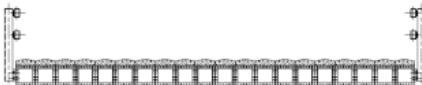
Figure 6 Fibre Composite Bridge Deck
