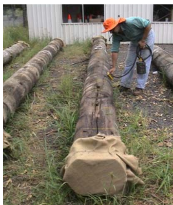
Figure 7 - GPR investigation of Purga Creek Girders
