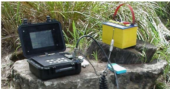
Figure 6 - SIR2000 control unit powered by a car battery
